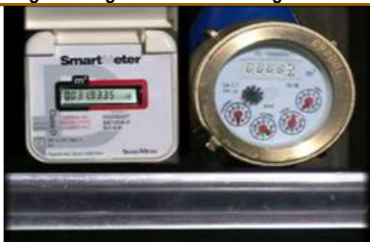
Figure 7: Water usage reading will be less due to grit and sand
